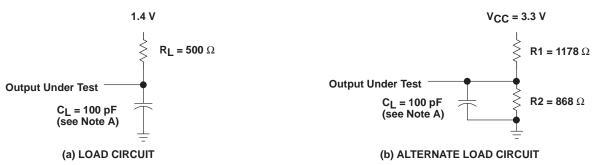
NOTE A: CL includes probe and fixture capacitance.
