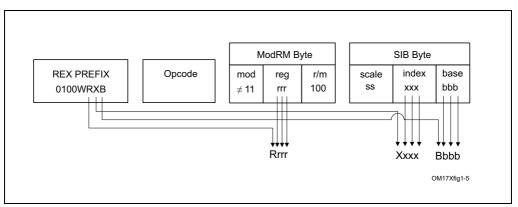
Figure 2-6. Memory Addressing With a SIB Byte
