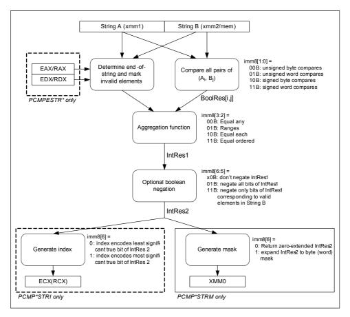
Figure 3-3. Operation of PCMPSTRx and PCMPESTRx
