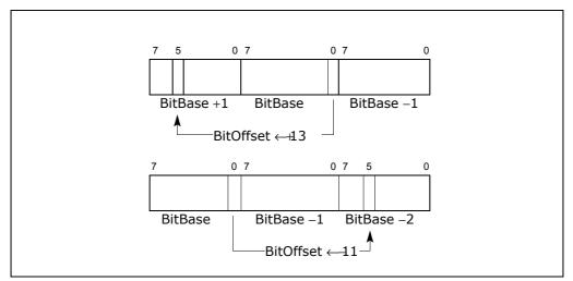
Figure 3-2. Memory Bit Indexing
