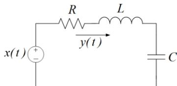
$$\frac{d^2 y(t)}{dt^2} = \frac{1}{L} \left( -R \frac{dy(t)}{dt} - \frac{1}{C} y(t) + \frac{dx(t)}{dt} \right)$$
